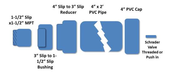
All Components Schedule 40 or 80 PVC Must be Pressure Rated NOT DWV (Drain Waste Vent)
