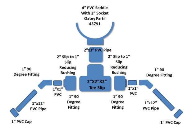
Working with compressed air and PVC can result in hazardous if not deadly conditions. As part of my build, I made sure to use schedule 40 (80 would be better) pressure rated PVC. I also made sure that the PVC was rated for pressure and not "DWV" (Drain Waste Vent) which is not pressure rated. The DWV pipes are typically marked in black ink and have "Not for Pressure" marked on them. PVC will fragment if it fails under pressure and can cause severe injuries and or death!
