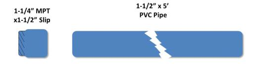
All Components Schedule 40 or 80 PVC Must be Pressure Rated NOT DWV (Drain Waste Vent)
