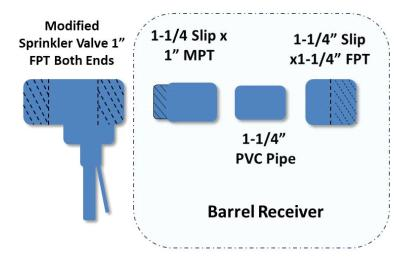
All Components Schedule 40 or 80 PVC Must be Pressure Rated NOT DWV (Drain Waste Vent)
